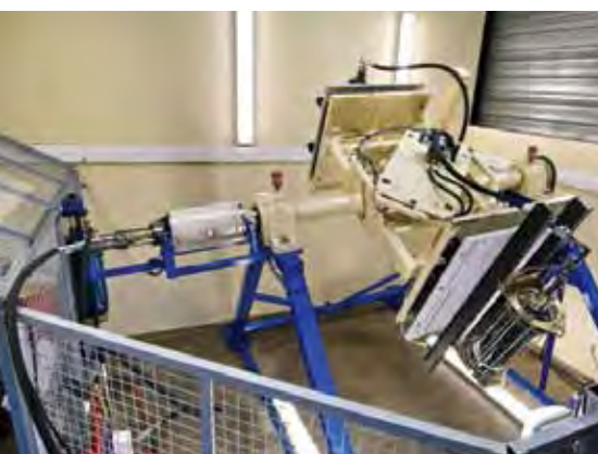
Accumulator test bench for wind turbine application.
