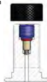
Model of valve stem integrated 5/8" 18 UNF (D)
