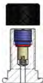
Model of valve stem integrated 7/8"14 UNF (C)
